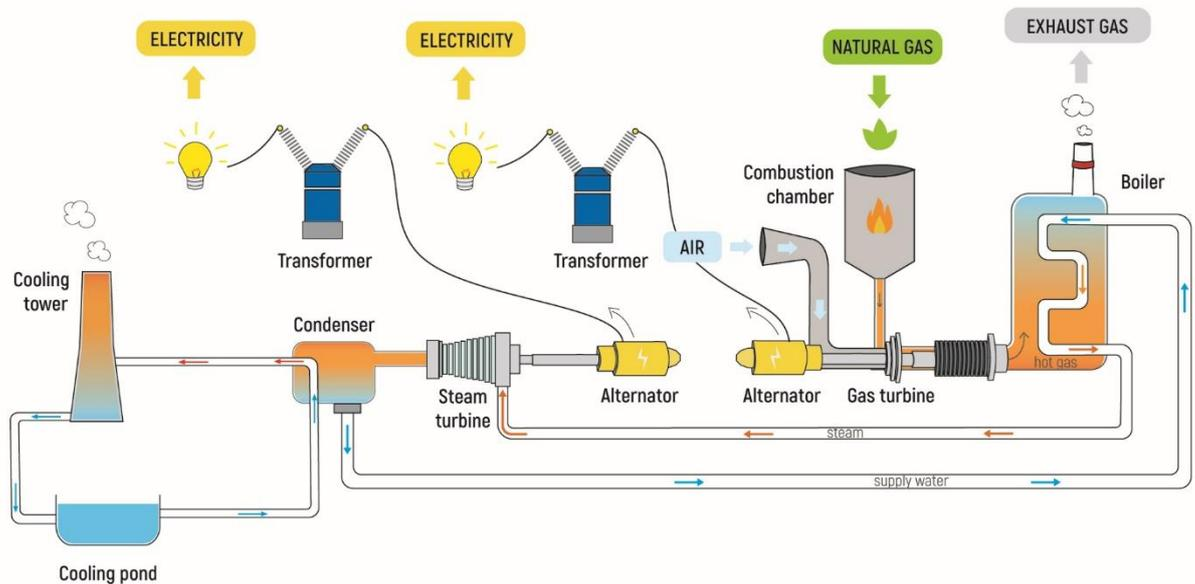
Figure 4-1. Generic Illustration of a Gas-to-Power Plant
