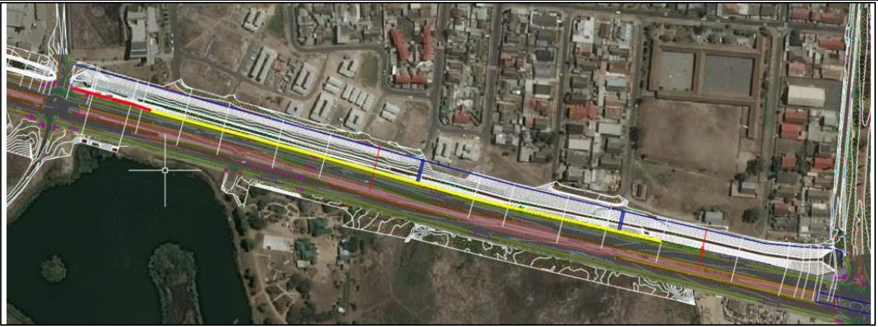
Figure 3 Encroachment into the Lotus Canal (yellow indicates where the proposed sidewalks would encroach by approx 3m and the red reaches indicate where encroachment would be up to 6m), the first nearby the Edith Stephens Wetland Nature Reserve and the second under the upstream pedestrian bridge (Source: GIBB, 2021)
