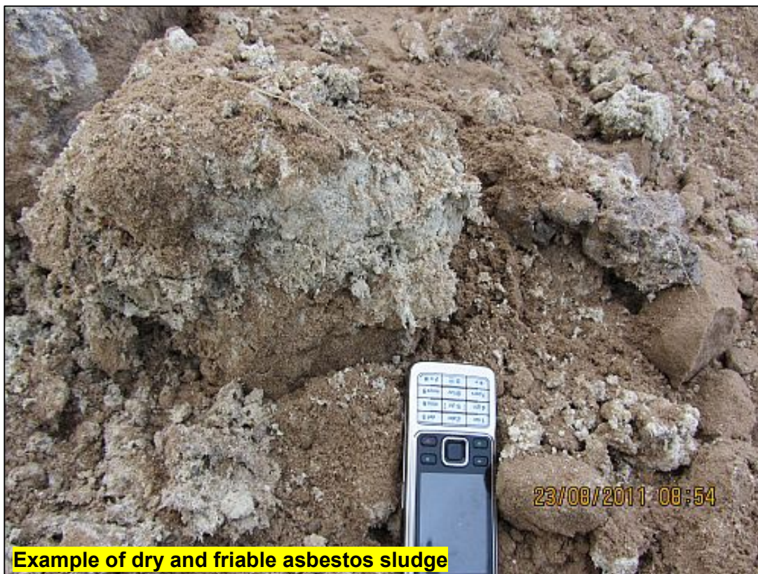
Two views of mixed asbestos wastes with little soil cover in the lower platform area. Note poorly compressed nature of the material.
