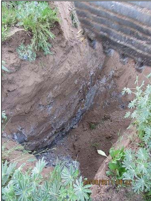
View of asbestos dry and friable sludge waste close to surface with little cover in lower platform area. Susceptible to mole disturbance.
