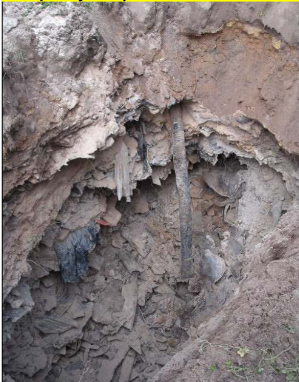
Two views of mixed asbestos wastes with little soil cover in the lower platform area. Note poorly compressed nature of the material.
