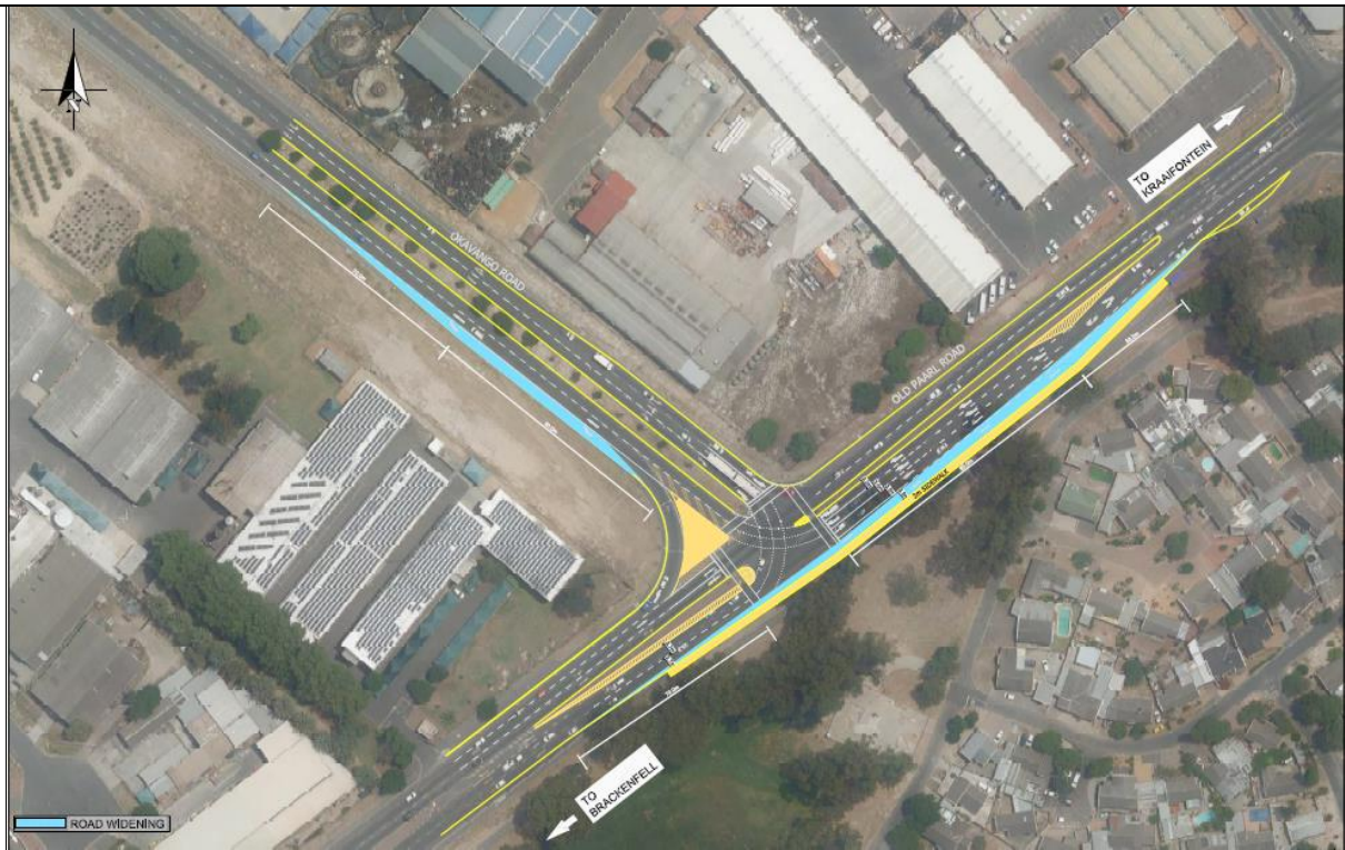
Figure 15: Proposed Upgrades at Okavango Road/Old Paarl Road Intersection (Source: Krogsheepers & Arangie, 2021)
