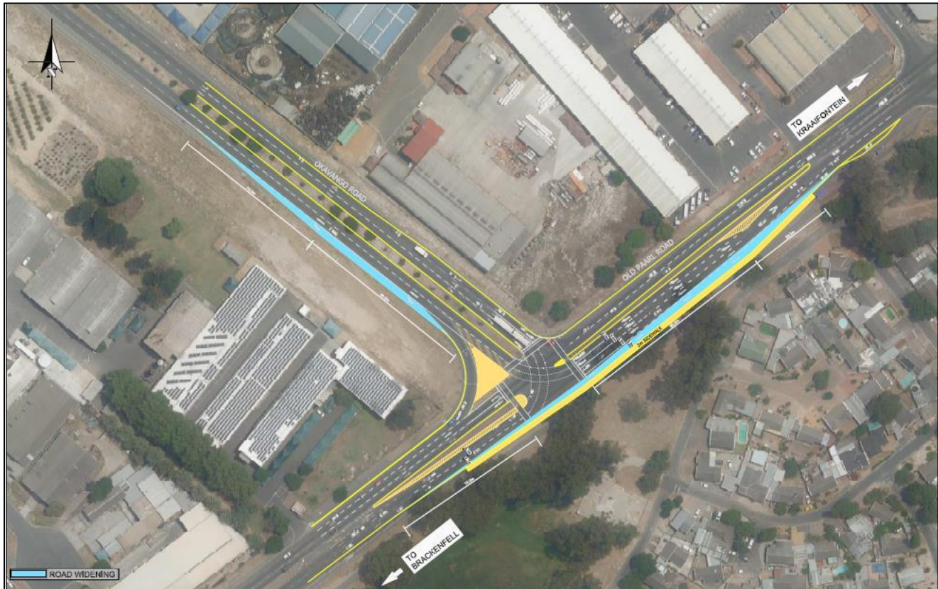
FIGURE 47: PROPOSED UPGRADES AT OKAVANGO ROAD/OLD PAARL ROAD INTERSECTION (SOURCE: KROGSHEEPERS & ARANGIE, 2021)
