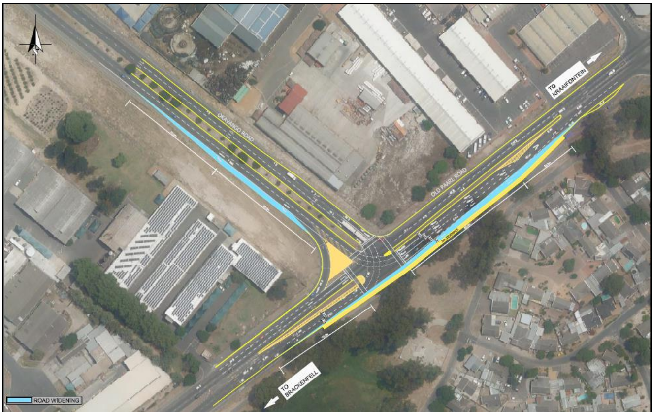
FIGURE 20: PROPOSED UPGRADES AT OKAVANGO ROAD/OLD PAARL ROAD INTERSECTION (SOURCE: KROGSHEEPERS & ARANGIE, 2021)
