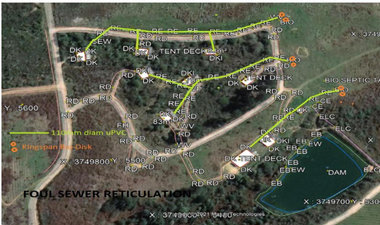
Figure 7.2 Sewer reticulation system at the Tented Camp site.
