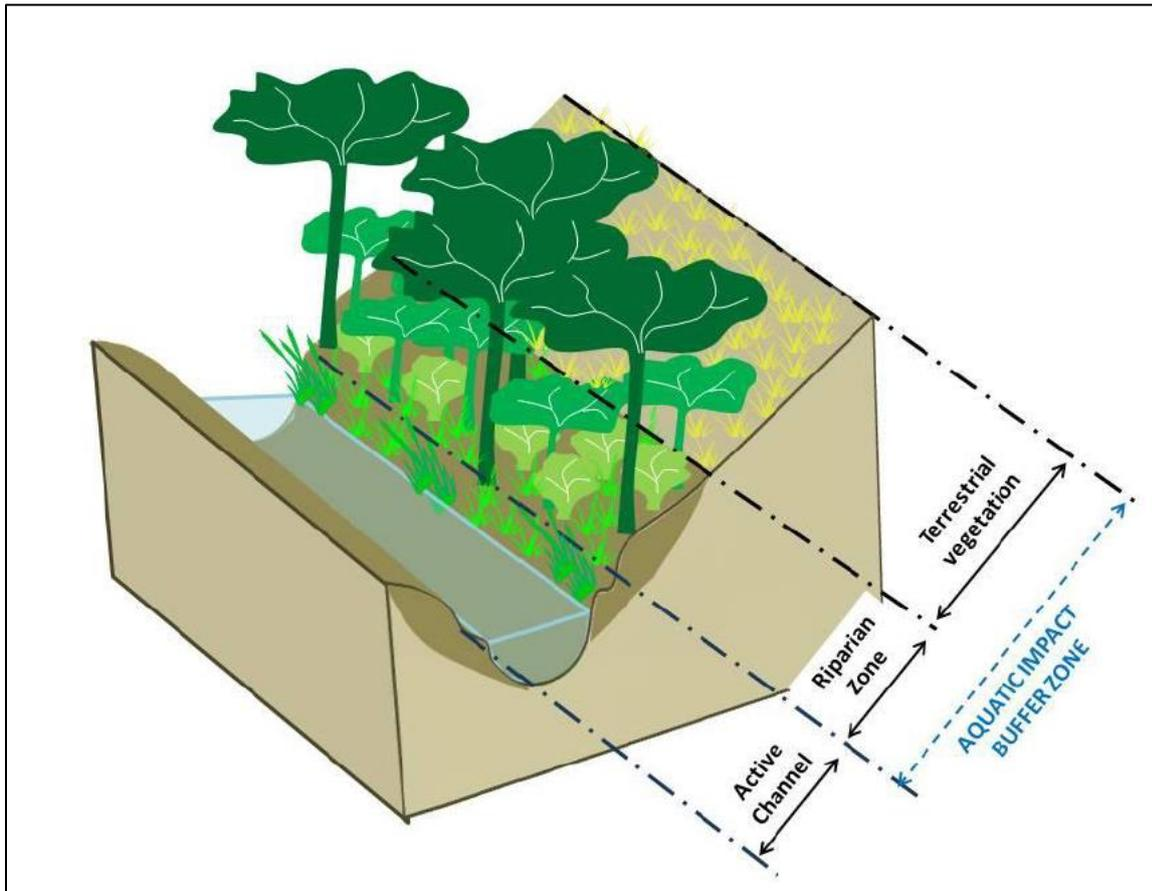
**Figure 1.2** Schematic diagram indicating the boundary of active channel and riparian habitat, and the areas potentially included in an aquatic impact buffer zone (MacFarlane and Bredin, 2016). The buffer (measured from the edge of the active channel) protecting a watercourse must include the riparian zone, and can extend into terrestrial vegetation.
