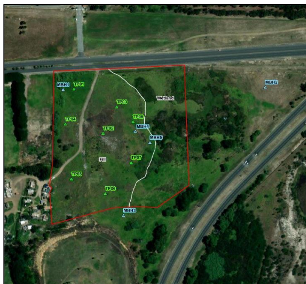
Figure jj. Monitoring boreholes (blue), extent of waste fill (white line) and excavation pits (green)
