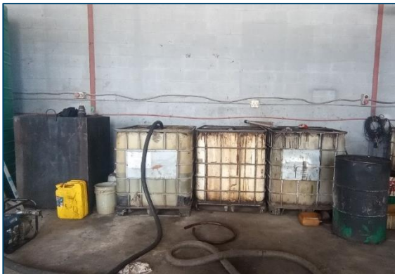
Figure 5: IBC tanks stored within a roofed structure on site.
