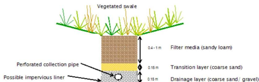
Figure 2: Bio-retention swale
